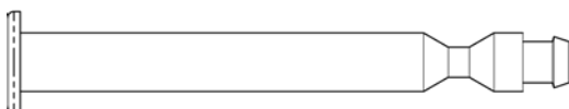
End Pin (scale 1:1) SH-PIN-END Finished in Black ONLY (NOTE: This pin is only used when placed next to a panel, cubby or cupboard)
